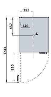
★ Main power cable▲ Drain pipe ø 31
