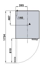
★ Main power cable▲ Drain pipe ø 31
